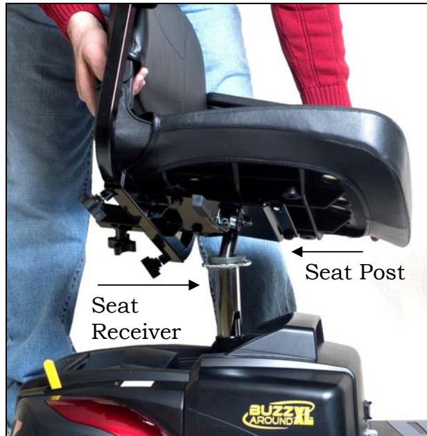
Figure 23. Installing the Seat
