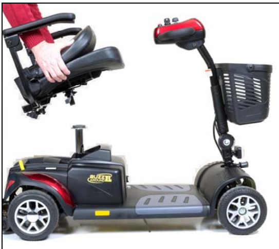
Figure 14. Removing the Seat
