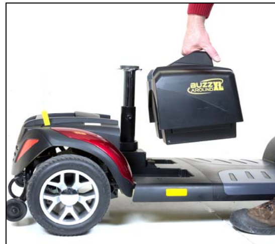
Figure 15. Removing the Battery Pack
