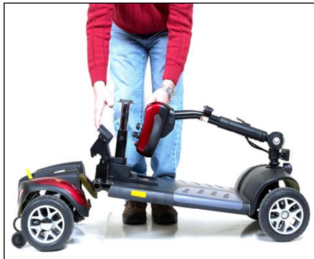
Figure 20. Connecting Frame and Drivetrain
