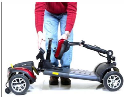
Figure 17. Separating the Drivetrain and Frame
