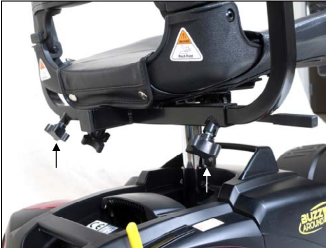
Figure 6. Armrest Width Adjustment
